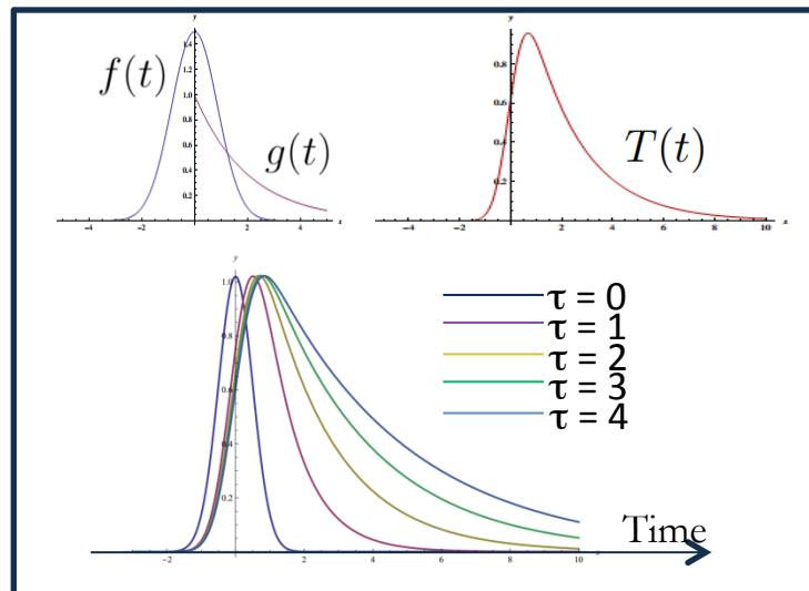
$$f(t) = Ae^{-\frac{(t-c)^2}{2\sigma^2}} \quad g(t) = \Theta(t)Be^{-\frac{t}{\tau}} \quad \left. \begin{array}{l} (f * g)(t) = \int_{-\infty}^{\infty} f(z)g(t-z)dz \end{array} \right\}$$
