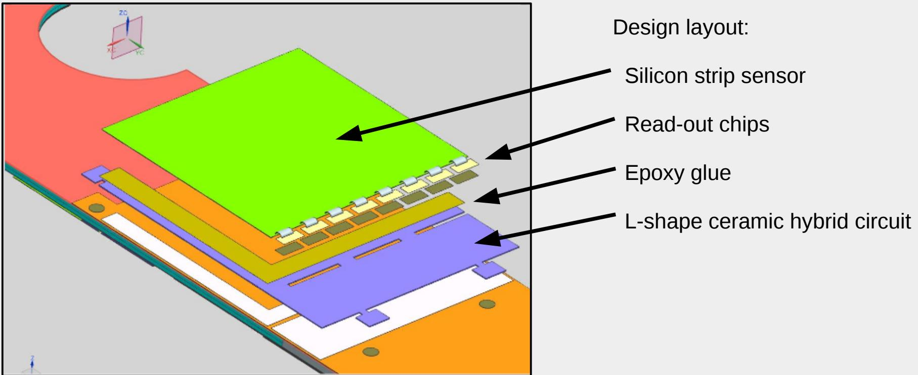
**Innovative solution**, based on **advanced ceramic** materials allows compact module design :
