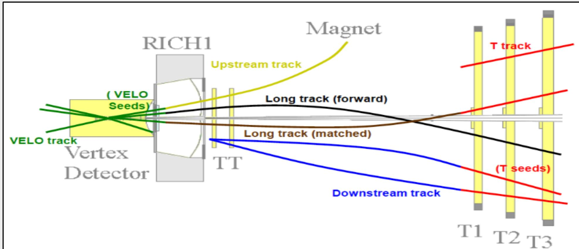
**Vertex Locator** → measures particle trjectories near the proton-proton interaction point
