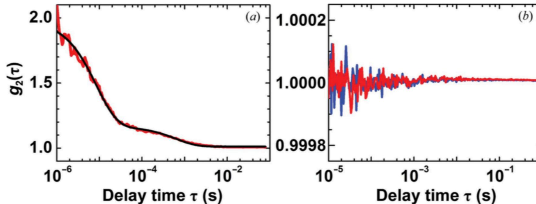
(a) A DLS intensity correlation function (red) of a lysozyme solution at 138 mg/ml in 20 mM NaAc buffer pH 7.8 and the fitted function (black). (b) cDDLS intensity correlation functions of the same lysozyme solution (red) and water (blue).
