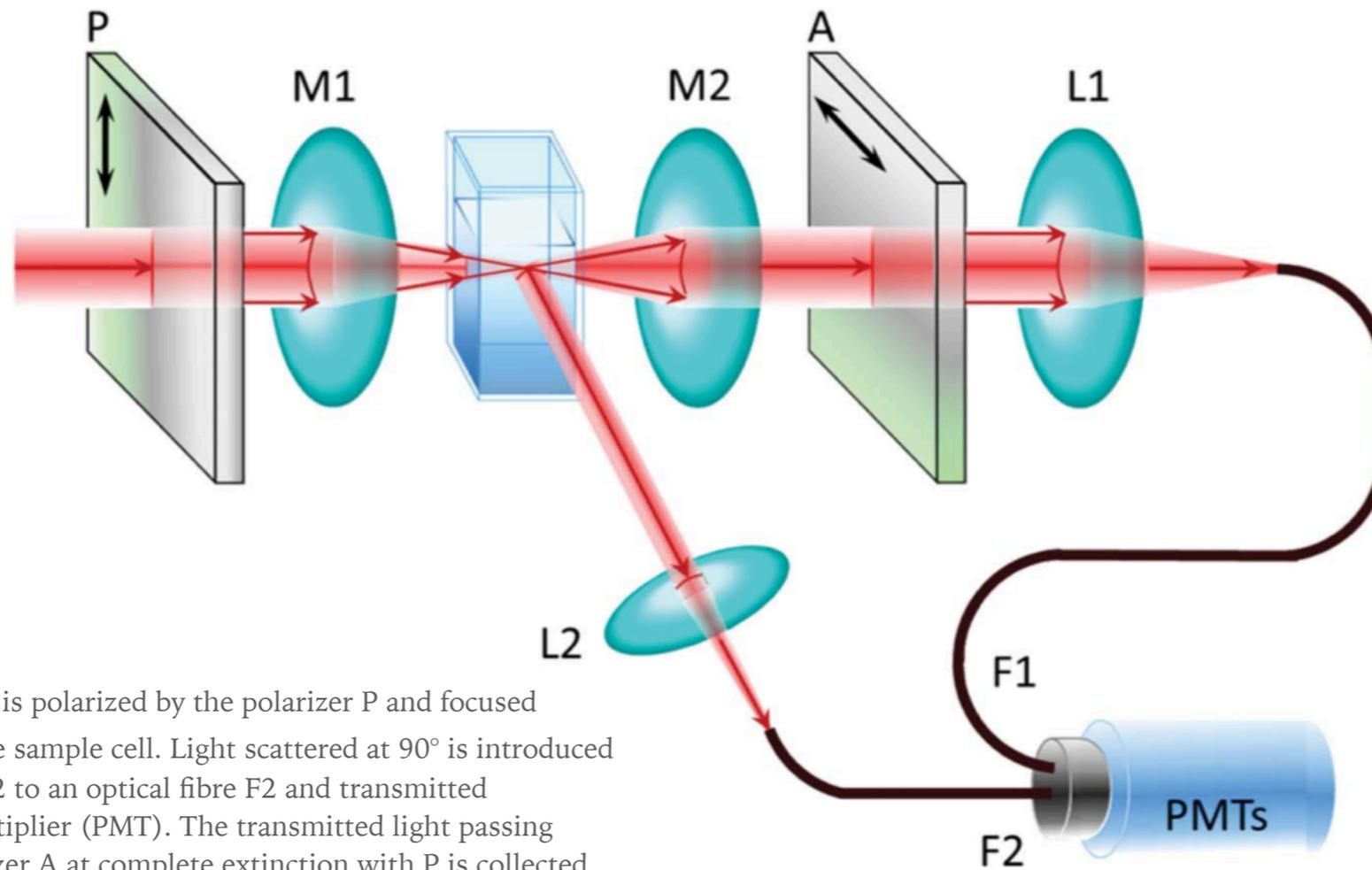
A laser beam is polarized by the polarizer P and focused by lens M1 into the sample cell. Light scattered at 90° is introduced by lens L2 to an optical fibre F2 and transmitted to a photomultiplier (PMT). The transmitted light passing through an analyzer A at complete extinction with P is collected by lens L1 in a confocal scheme and sent by optical fibre F1 to a second photomultiplier. Both PMTs are connected to correlators.
