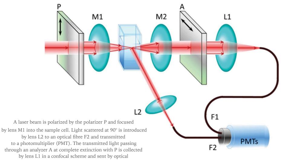
fibre F1 to a second photomultiplier. Both PMTs are connected to correlators.
