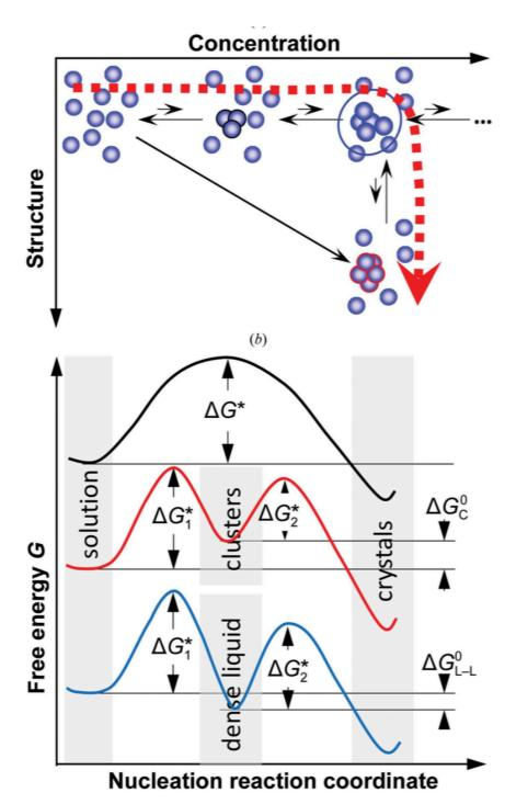
The two-step mechanism of nucleation of crystals.
