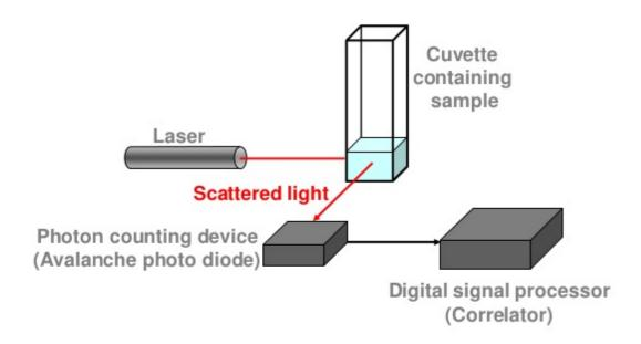
Dynamic light scattering refers to measurement and interpretation of light scattering data on a microsecond time scale.
