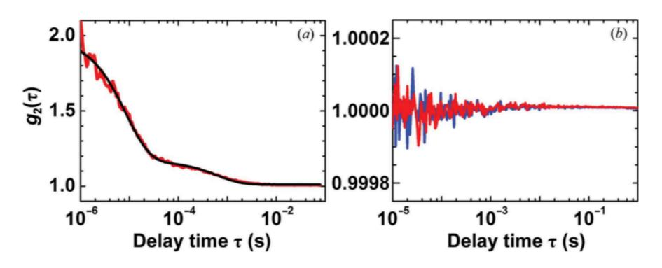
(a) A DLS intensity correlation function (red) of a lysozyme solution at 138 mg ml in 20 mM NaAc buffer pH 7.8 and the fitted function (black). (b) cDDLS intensity correlation functions of the same lysozyme solution (red) and water (blue).
